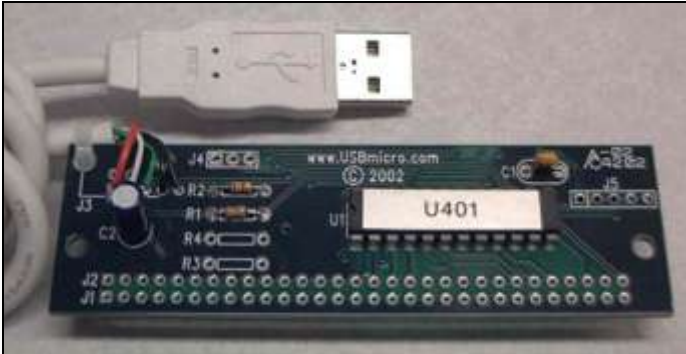
Figure 2.7: This U401 I/O board from USBmicro is fully supported by RobotBASIC.
