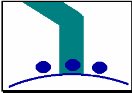
Figure 7.2: The Line-Sensors Setup In RobotBASIC
