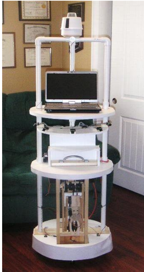
Figure 12.20: Note the high-mounted beacon detector.
