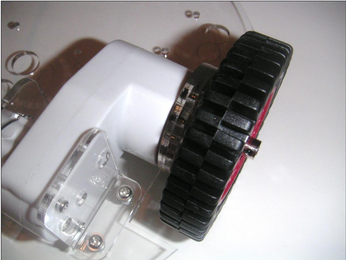
Figure E-7: The holes in the wheel should match the donuts mounted on the plates. A collar with a set screw holds the wheel in place.
