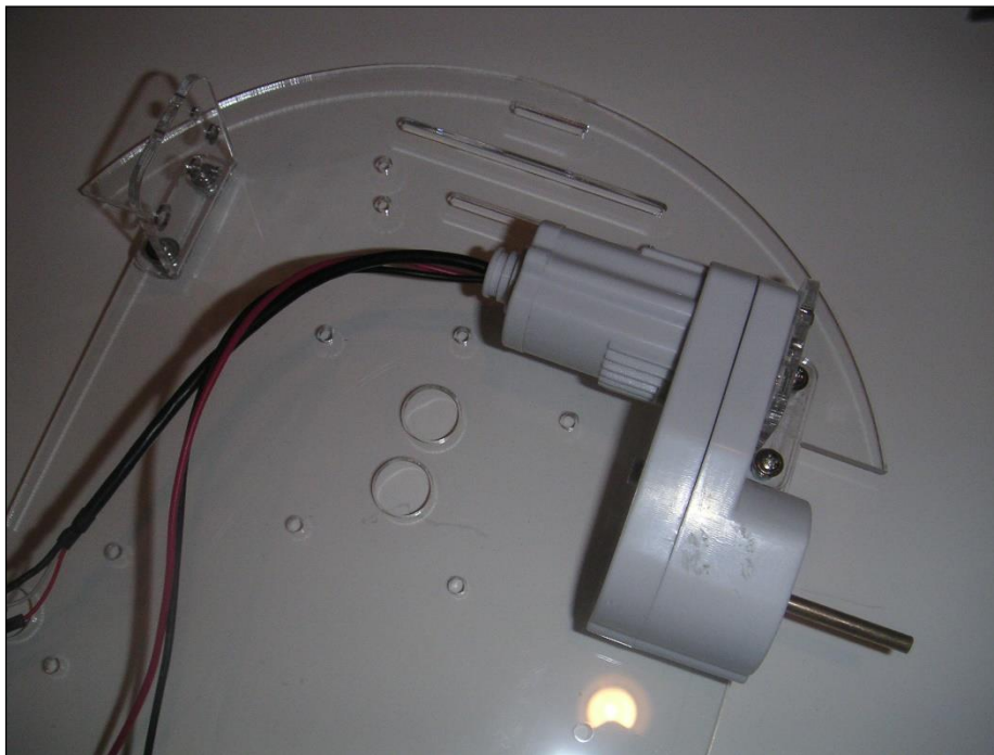
Figure E-2: Mount the outside motor brackets as shown.
