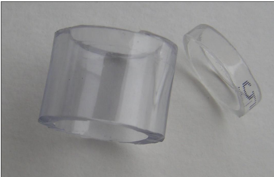
Figure D-9: Two small pieces of rubber tubing can be used to make a hooded shield.
