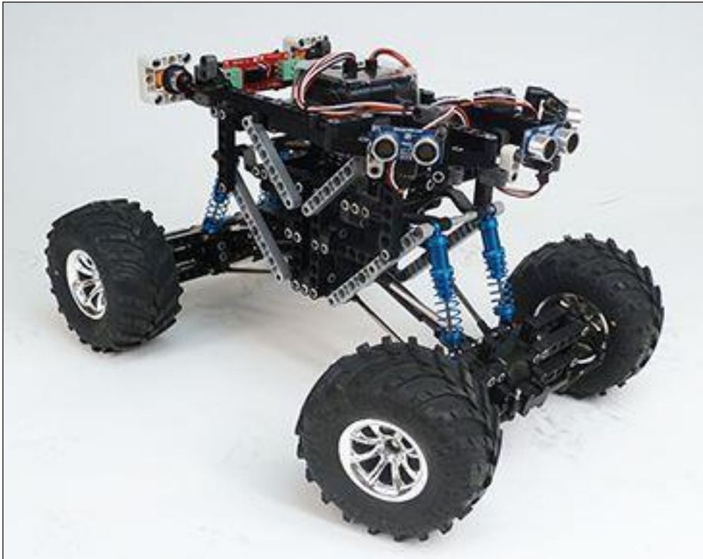
Figure 7.1: Steerable robots, such as this all-terrain vehicle from MINDS-i offer increased stability in an outdoor environment.
