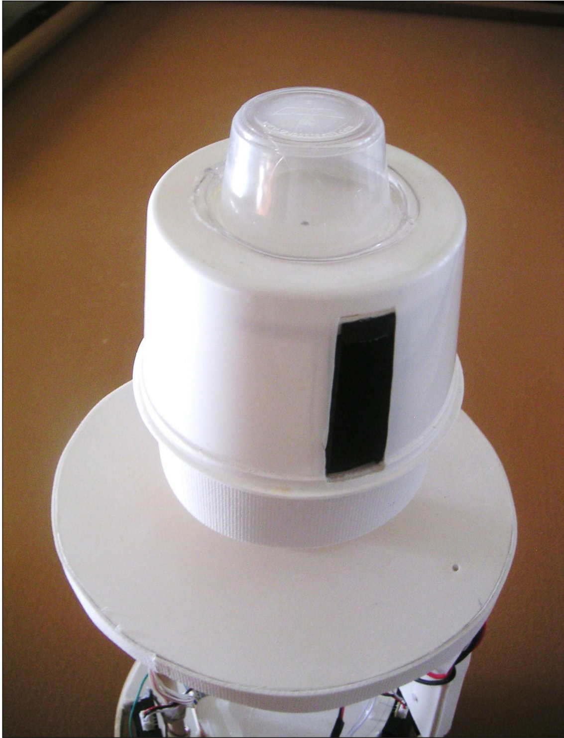
Figure 13.2: Our Nav-Assist assembly supports both narrow and wide slit beacon detectors that are rotated by a small servomotor.
