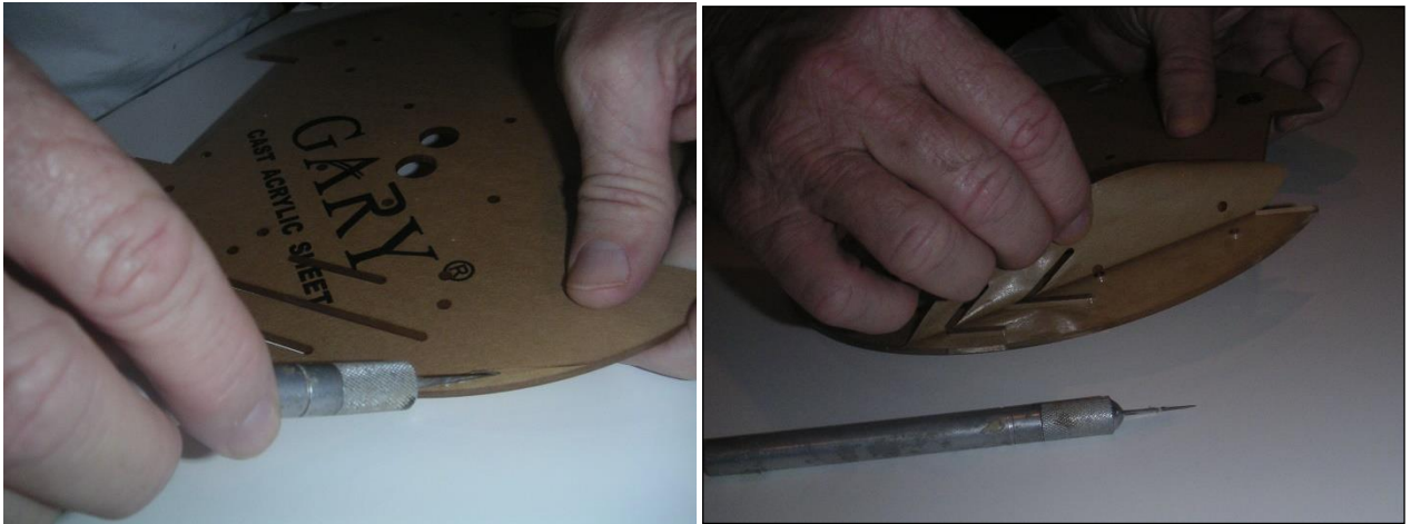
Figure E-2: Remove the protective paper from all plastic parts.
