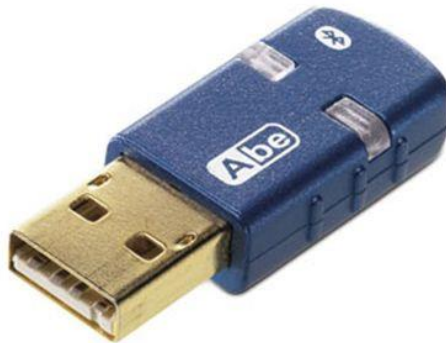
Figure 1.6: When you plug a Bluetooth adapter into your PC's USB port, RobotBASIC can communicate wirelessly with the transceiver in Figure 1.4. There are no wires to your robot and no programs to download. Just run your RobotBASIC program on the PC and the robot responds.
