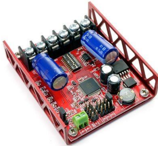
Figure 5.1: RoboClaw controllers allow the RROS to control large motors.
