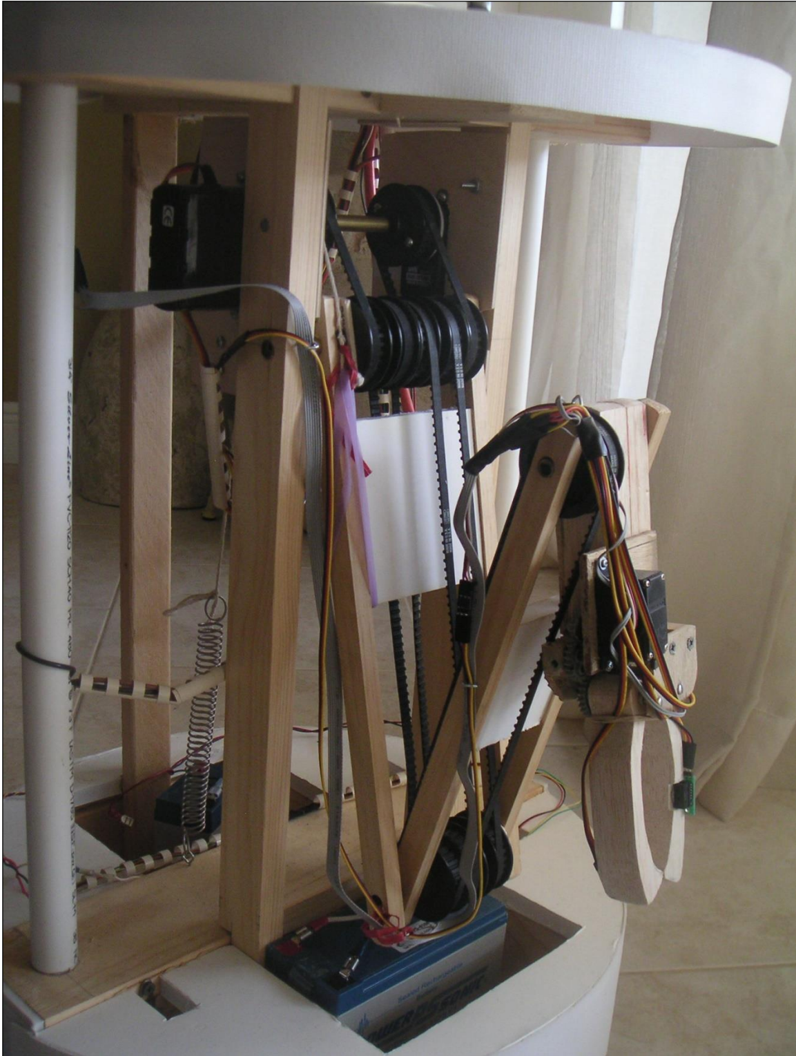
Figure 15.9: The arm folds into the body when not in use.
