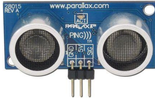
Figure 9.6: The Ping ranging sensor can be read with a digital pin.
