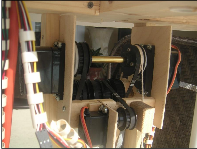
Figure 15.10: All joint motors are mounted behind the arm.
