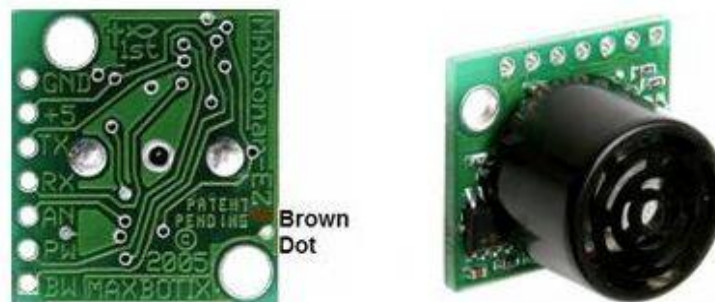
Figure 9.7: The Maxbotics ranging sensors have an analog output mode that the RROS will support.
