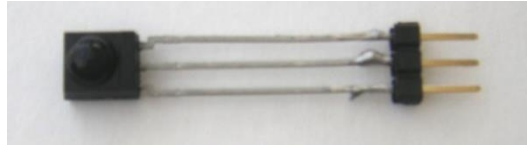
Figure D-7: A 3-pin male header is soldered to the beacon detector.
