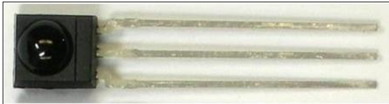
Figure 12.3: This small device serves as a beacon detector.
