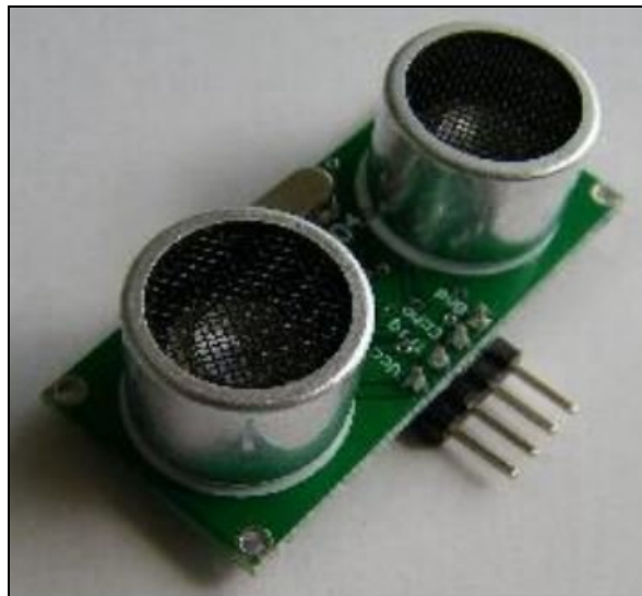
Figure 3.1: This ranging sensor can measure the distance to nearby objects.
